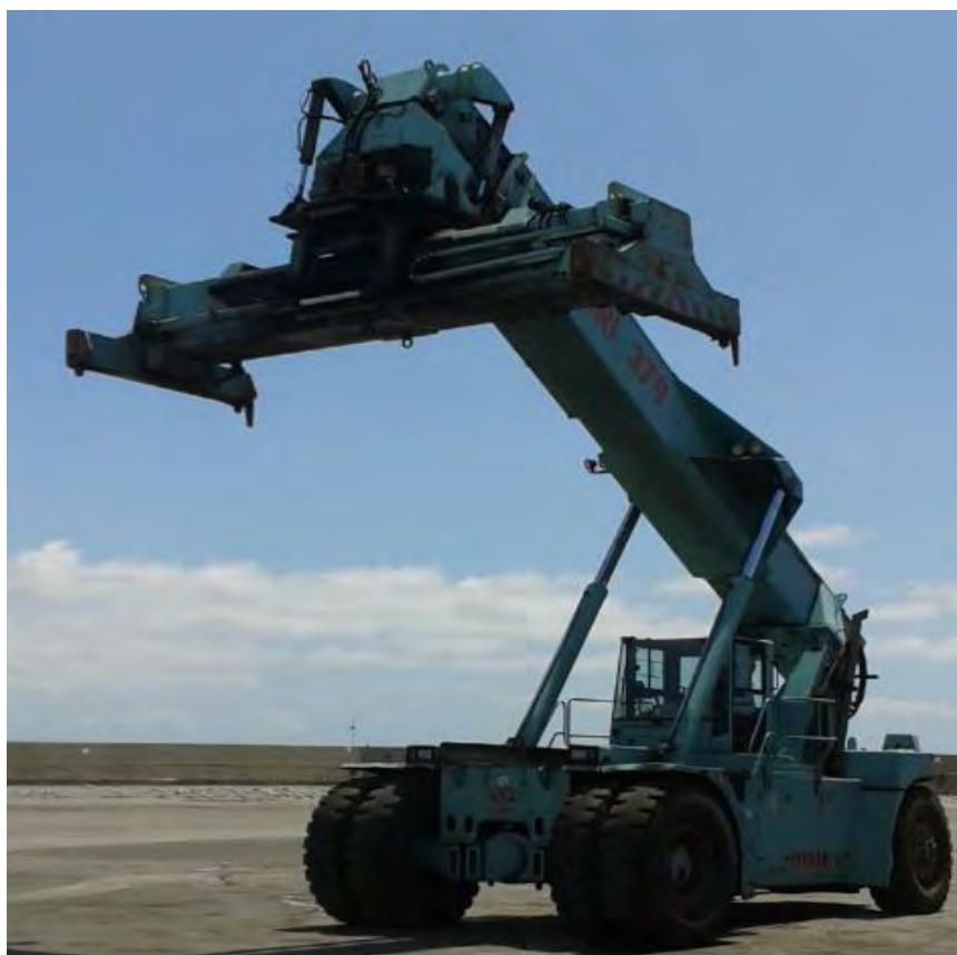
Fig. 2.7 - Reach stacker in piazzale
